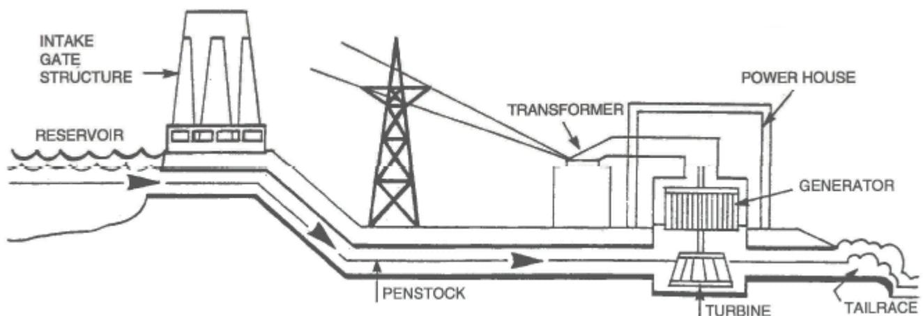
**The flow of water in a hydroelectric station**
